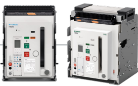
기중차단기 · AC : up to 150 kA, 6,300 A up to 130 kA, 6,000 A (UL1066, ANSI C37.13/16/17/50, CSA C22.2 no. 31) · DC : up to 60 kA, 4,000 A
